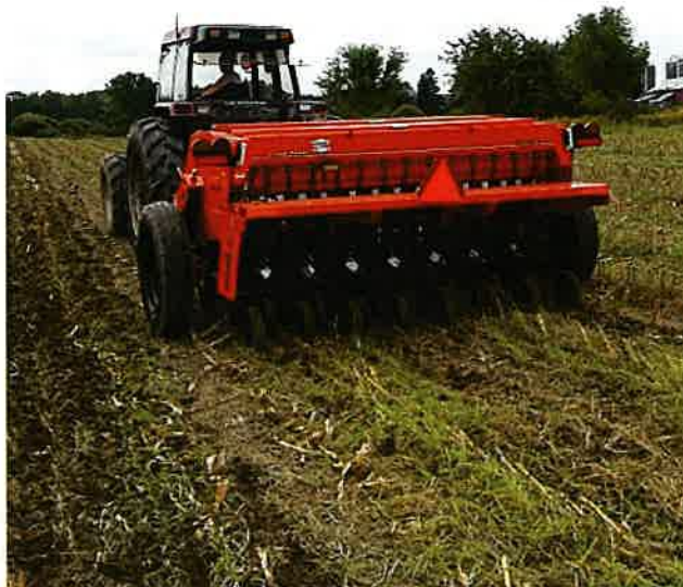
A no-till drill is used in Erie County to plant cover crops in the existing post-harvest crop residue.
