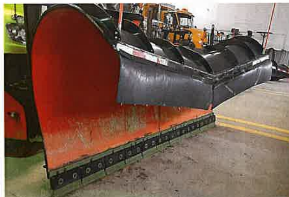
Left: Plow with adaptive blade retrofit to help remove ice from the road, using less salt. Right: Road temperature sensor to better gauge when to apply salt reducing the amount applied.
